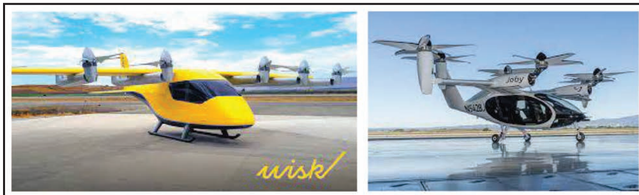
Figure 12. Wisk Aero (“Wisk”) all-electric, autonomous four seat eVTOL (electric vertical takeoff and landing) flying taxi
